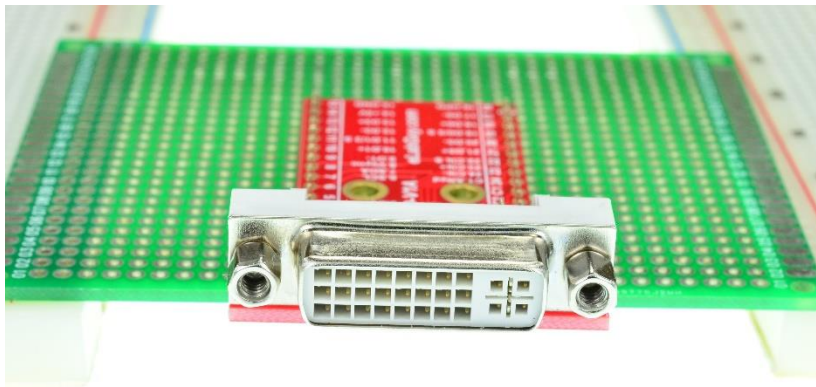
Figure 4: Solid Mounting on prototype PCB
